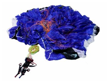
Step 1: Bundle up your glider in form of a cabbage. This way you're avoiding that the glider drags over the ground during folding.
