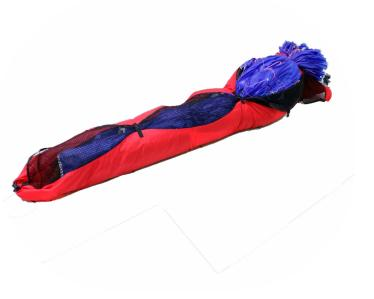
Step 5: At last fold the sack as shown in the photo. This method is very gentle to the more stiffer parts of the glider.
