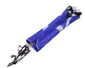
Step 5: Fold the sack as shown in the photo. This method is very gentle to the more stiffer parts of the glider.
